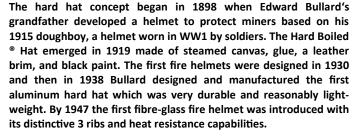
The evolution of the hard hat has continued with thermoplastics which is lighter and less costly. In 1982 the hard hat changed again with the introduction of the non slip ratchet suspension and as with
