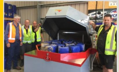
McFall Fuel has recently purchased a washer, pictured above, to speed up the time consuming process for the Lubricant Logistics Team. The Apollo Power Washer holds 14 x 20 Litre instead of 4 per cycle. The waste oil and the containers to be recycled are collected by bona fide operators. The containers for reuse become part of the McFall Fuel Reuse & Recycle Programme.
