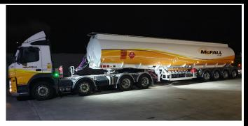
fleet since 2015 with the merges with Direct Fuels and then Rural Fuel. The new quad pictured was developed as part of the drive to have a fit for purpose heavy fleet to meet the wide range of needs across the North Island. The four axle 6 compartment is able to carry 37,000 litres of motor spirits and 32,000 litres of diesel at 44 tonne.
